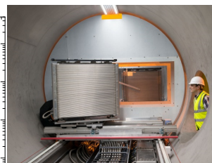
Two 1m square detectors in a 13m long, 3.25m diameter vacuum tank.
